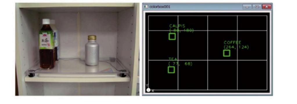
Fig. 7. Information about objects provided by the intelligent cabinet. Squares on the screen indicate the position of the different objects together with their description.
