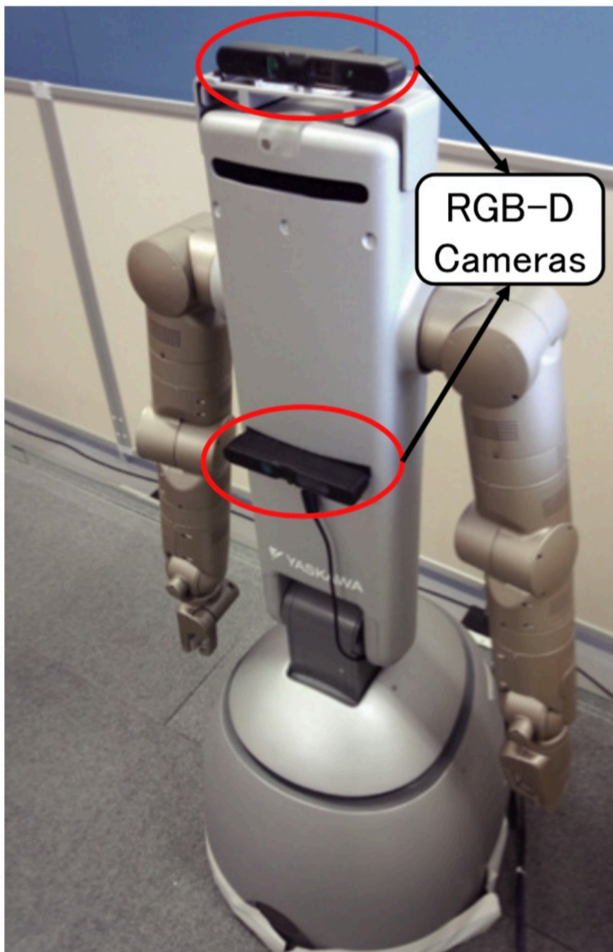
Fig. 8. SmartPal-V is equipped with two RGB-D cameras.
